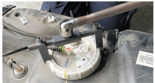
Photo 5a: Remove pickup unit
